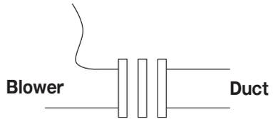
When using the heat-resistant model with [ **intake air temperatures of 60°C or greater** ], be sure to take [ **thermal expansion** ] into consideration and use heat-resistant fittings to prevent heat expansion of the ducts.
