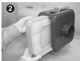
2 Slide the filter box to take it out.
