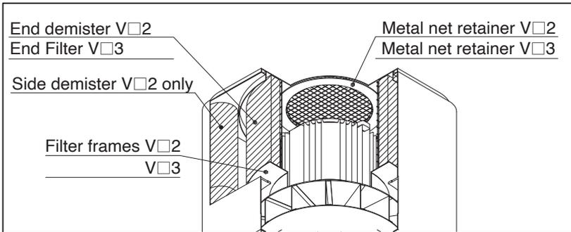
(3) Internal component names and layout for CRH Series Mistresa
