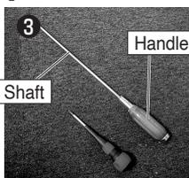
To detach the outer cylinder and install the filter frame, use a long screwdriver (200 mm or longer shaft). Smaller screwdrivers may not reach the screws if the handle gets stuck in the opening.
