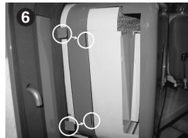
When installing the cap after replacing the filters, be sure to put the guide into the guide slot. Otherwise, improper installation of the cap could lead to oil leak.
