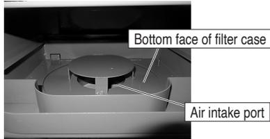
**If cutting chips are sucked into the unit**
