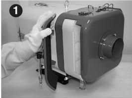
1 Unclamp the filter. Remove the cap.
