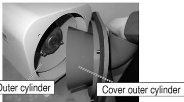
Remove the screws that lock down the side cover and detach the side cover so that the outer cylinder on the main body side and cover outer cylinder on the side cover side are visible.
