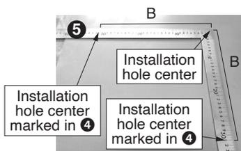
Mark the centers of the remaining installation holes (x 2), at the distances from the installation holes marked in 4 specified in the installation dimensions on pg. 2.
