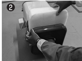
Remove the front demister (front filter).
