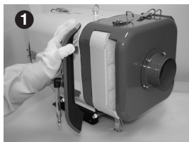
Unclamp the filter. Remove the cap.
