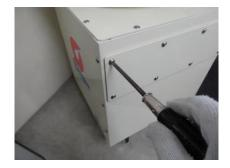
Insert the filter box with the demister facing down toward the main body of the machine and screw it in with truss head screws using a cross slot screwdriver. (Eight locations)
