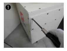
Remove the truss head screws on the filter box using a cross slot screw driver. (Eight locations)
