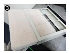
Withdraw the demister (one sheet) and the filters (three sheets) from the filter box
